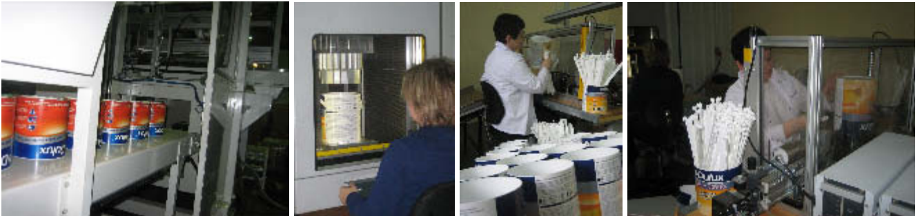
Paintainer is moulded and decorated with IML in a fully automated process. Next step is welding the ring and mounting the handle.
